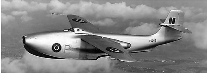
The Saunders-Roe SRIA1 jet fighter flying boat was powered by two Metrovick F214 Beryl engines and first flew on 16 July 1947.
